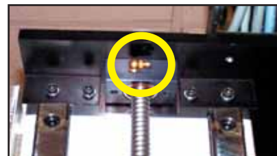
Z-AXIS END BEARING
