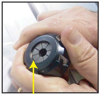
This picture shows an improper assembly. Notice the gap and angle of the collet in relation to the nut. The collet is not flush to the end of the collet nut. Correct this assembly before using.
