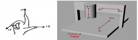
Fig. 2 1 Coordinate system abiding by right-hand rule
