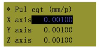
Fig. 5-7 Setting page of pulse equivalent
