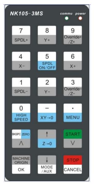
Fig. 4-2 Panel keys arrangement picture
