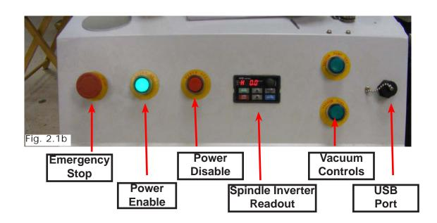
Once the main power switch has been engaged the controller is activated by pressing the green on switch on the front of the controller.
