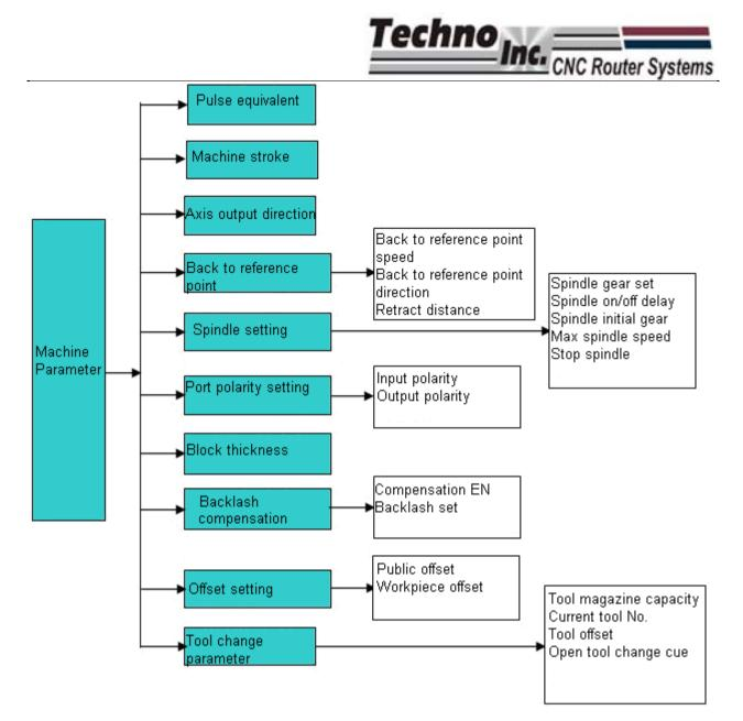
Fig. 5-6 Submenus of all different levels under machine parameter configuration page
