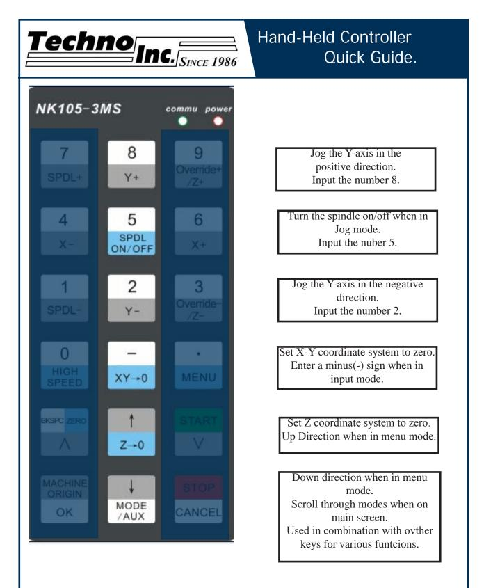
The Mode/Aux key is a special key that can be used in combination with other keys for various functions. The following page lists these functions.
