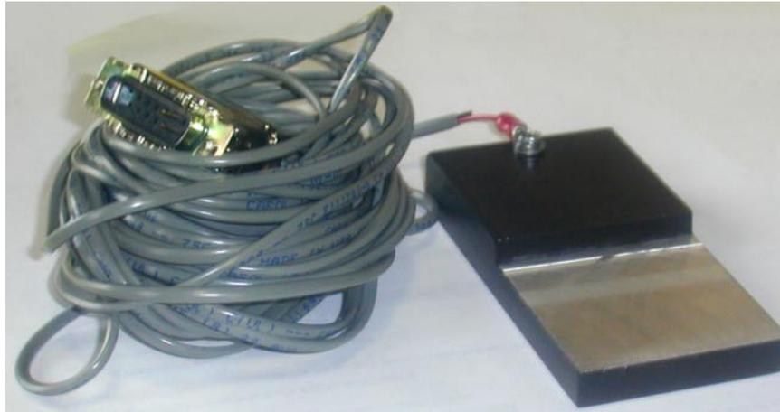
In this Tutorial we walk you through the important task of zeroing a tool (bit) on a workpiece. The Techno touchpad helps automate and calculate this process for you.
