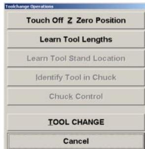
**NOTE:** Make sure that the tool bit is located directly above the touchpad (about 4 or 5 inches). Although, this is just a Tutorial, in the future it is likely you will be setting the top portion of your workpiece as the Z-axis zero. So, if you want to place the touchpad on top of some cutting material for this portion of the Tutorial, do so now.
