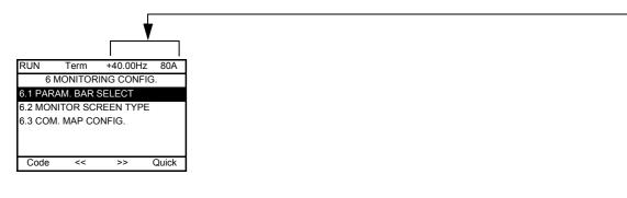
[6.1. PARAM. BAR SELECT]: Selection of 1 to 2 parameters displayed on the top line (the first 2 cannot be modified).
