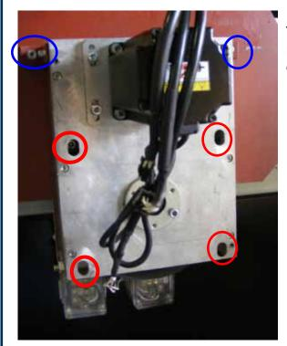
The motor on both sides on the Y gantry will need to be dropped so that the pinion is not engaged with the rack.
