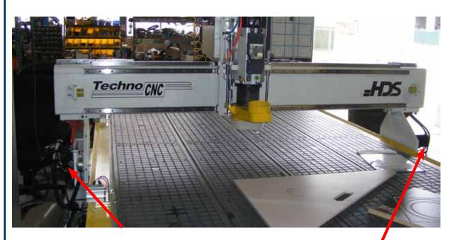
Disable power to the machine and remove the side panels from the Y axis motors, so that the Y-axis motors are exposed as above.
