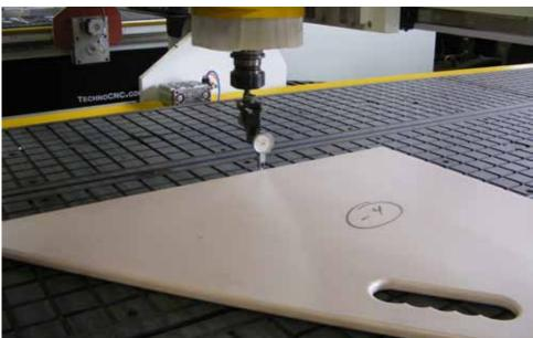
Adjust the precision square until there is little or no movement on the dial indicator as you jog it up and down in the Y-Axis.
