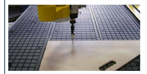
Using a rubber mallet lightly tap the gantry in the direction the machine needs adjustment.
