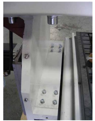
Loosen the 8 screws that hold the uprights to the bearing carriages.
