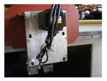
Engage pinion to the racks on both sides of the gantry and tighten all the screws.
