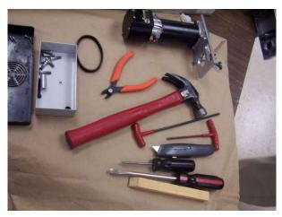
TOOLS: Hammer, M4, M5 Allen keys; wire-cutter, utility knife, Phillips Head Screwdriver, Large flat screwdriver, Blobk of wood
