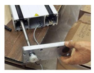
By pushing the ball screw from the opposite end of the slide (non-motor end) the casting can be removed as a complete assembly.
