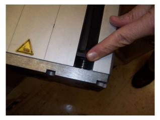
Slide the little plastic endpiece back to prepare to remove the end-casting
