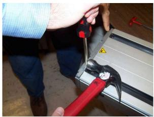
Use the wooden block (preferably not to scratch anything) or the screwdriver to remove the end-casting.
