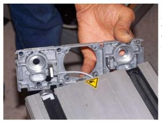
Once the castings is freed, the limit switch can be seen on the casting. If it is functioning properly then the limit switch on the motor end is faulty and the other X-axis end-casting will have to be removed.
