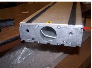
Remove the cap screws that hold the end-casting
