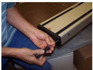
Remove the screws that hold on the cover from the non-motor end of the X-axis
