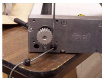
Remove the grommet from the cable as it enters the slide.
