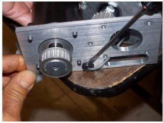
Pry off the cable grommets. These can be opened up and removed. And then finish removing the four screws that hold on the motor plate.
