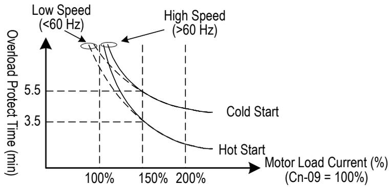
Fig. 36. Motor overload protection curve (Cn-09 setting = 100%)
