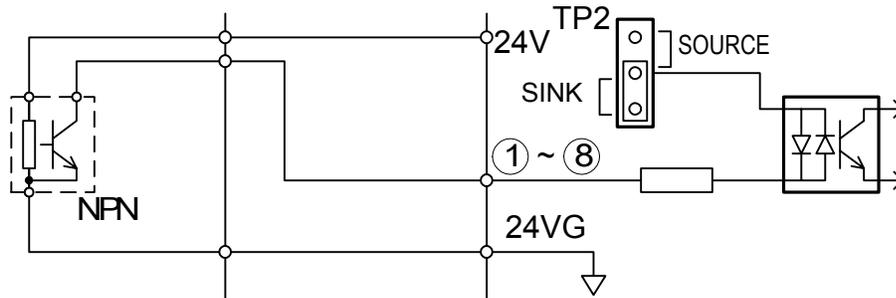
(b) SOURCE Type Input Interface : The short pin of TP2 is set to SINK position.
