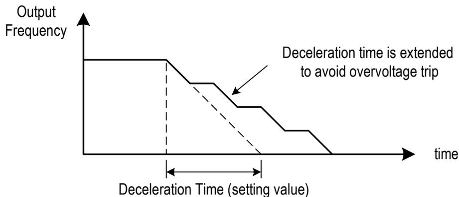
Fig. 34. Stall prevention function during deceleration (Sn-15= 1)
