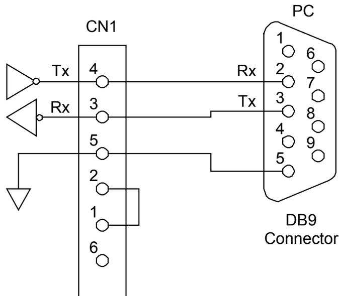
**Fig. 52. RS232-C Typical Connection Diagram**
