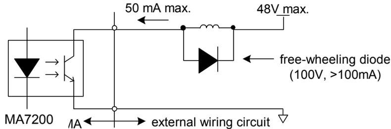
Fig. 4. The Optical-couplers connect to external inductive load
