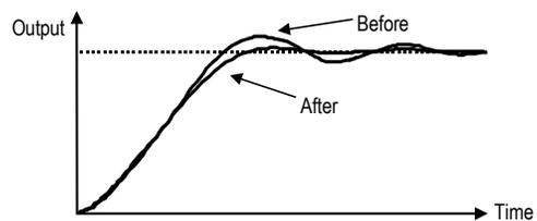
If oscillation occurs with a longer cycle than the integral time (I) setting, then the integral operation is strong. The oscillation will be reduced as the integral time (I) is lengthened.
