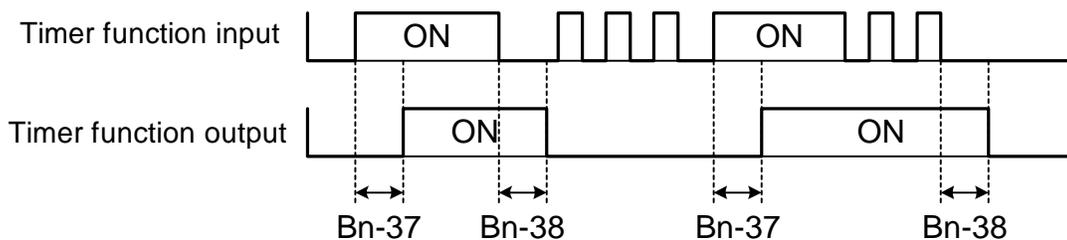
Fig. 15. An operation example of timer function
