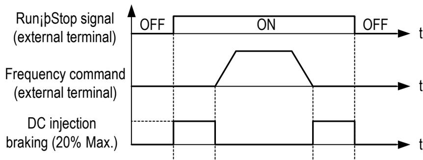
Fig. 35. Zero speed braking operation selection
