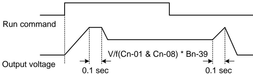
Fig. 16. Time chart for energy-saving operation
