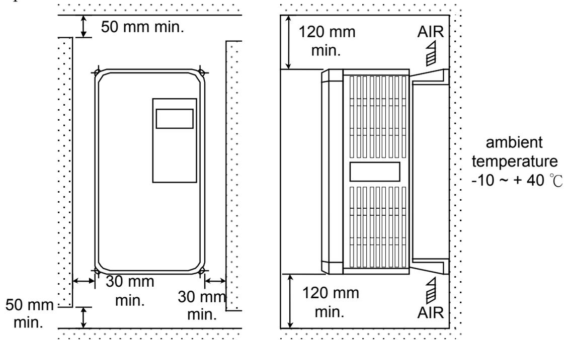
Fig. 1-a. Air clearance for MA7200 wall mounting
