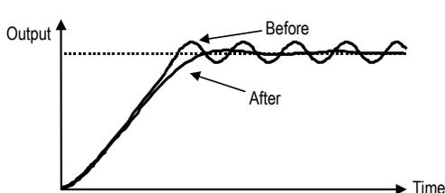
If oscillation cycle is short and approx. the same as the derivative time (D) setting, then the derivative operation is strong. The oscillation will be reduced as the derivative time (D) is shortened. If even setting the derivative time (D) to 0.00 cannot reduce oscillation, then either decrease the proportional gain (P) or raise the PID primary delay time constant.
