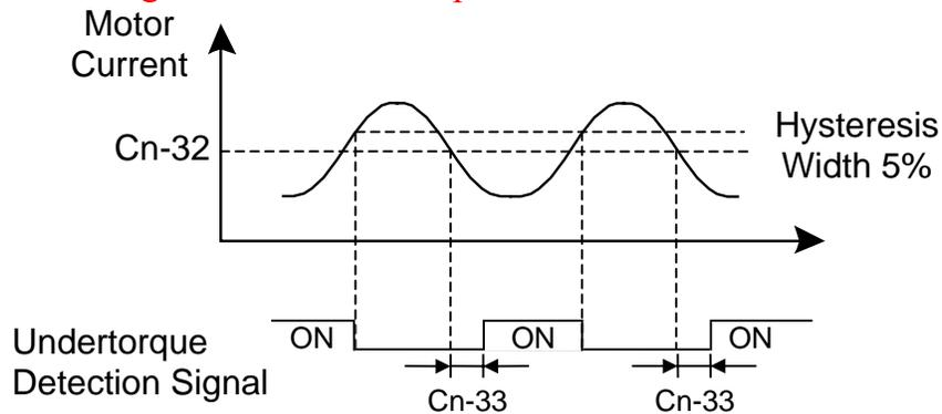
Fig. 25-b. Undertorque Detection Time Chart
