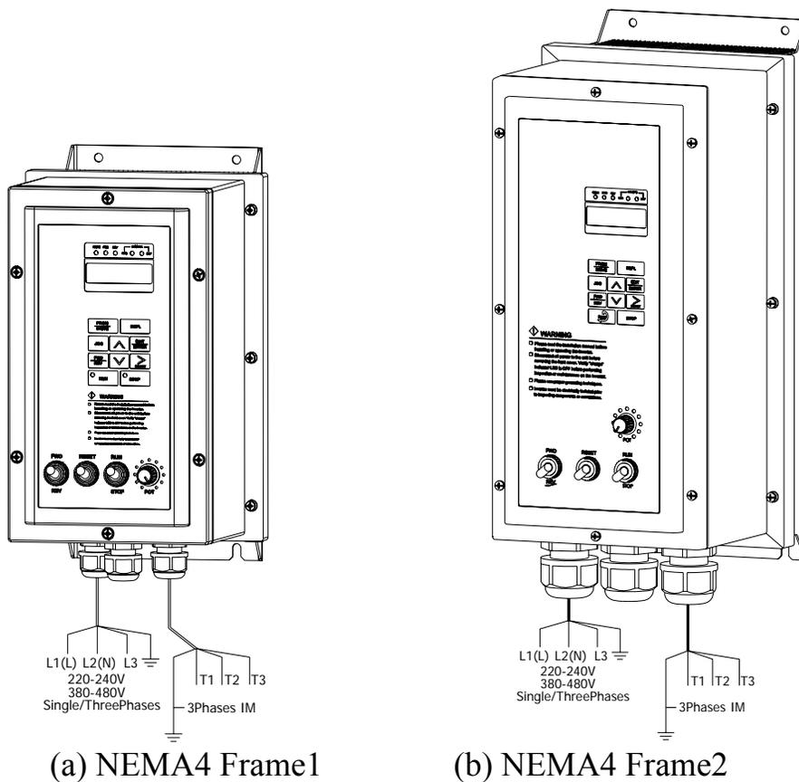
Fig. 1-b. MA7200 NEMA4 Installation
