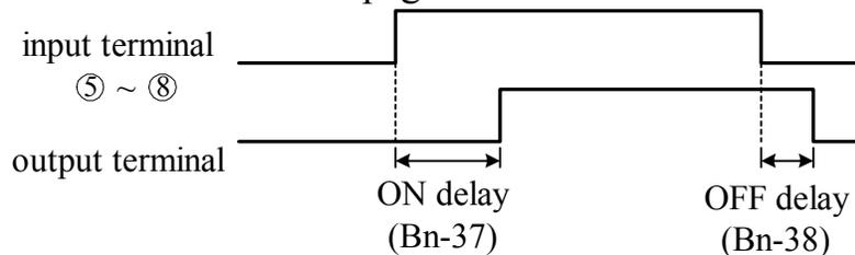
Fig. 46. The input/output signal in ‘Timer’ function application
