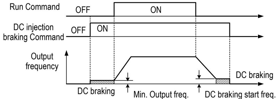
Fig. 42. Time chart for DC injection braking command
