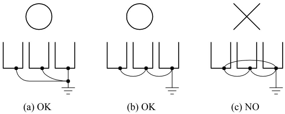
Fig. 5. MA7200 ground winding
