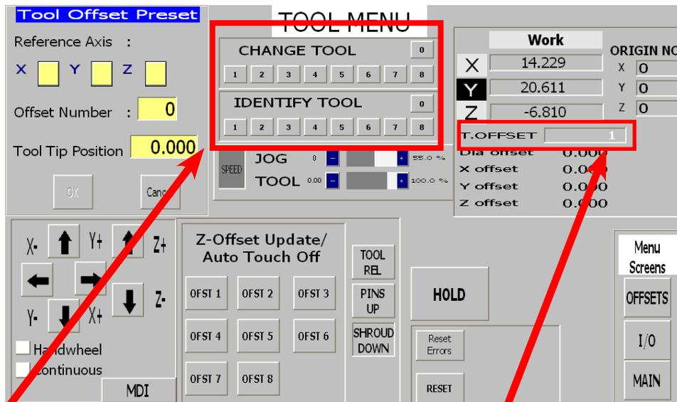
Identify or Change Tools by pressing these buttons. 0 is an empty chuck.
