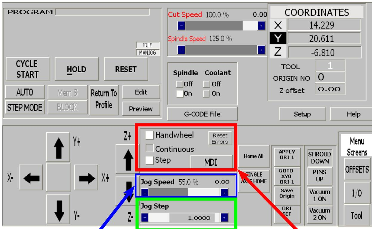
Increase or decrease the jog speed by pressing the blue +or- box. Speed is shown in % of maximum speed. Actually speed is displayed when the machine is running.
