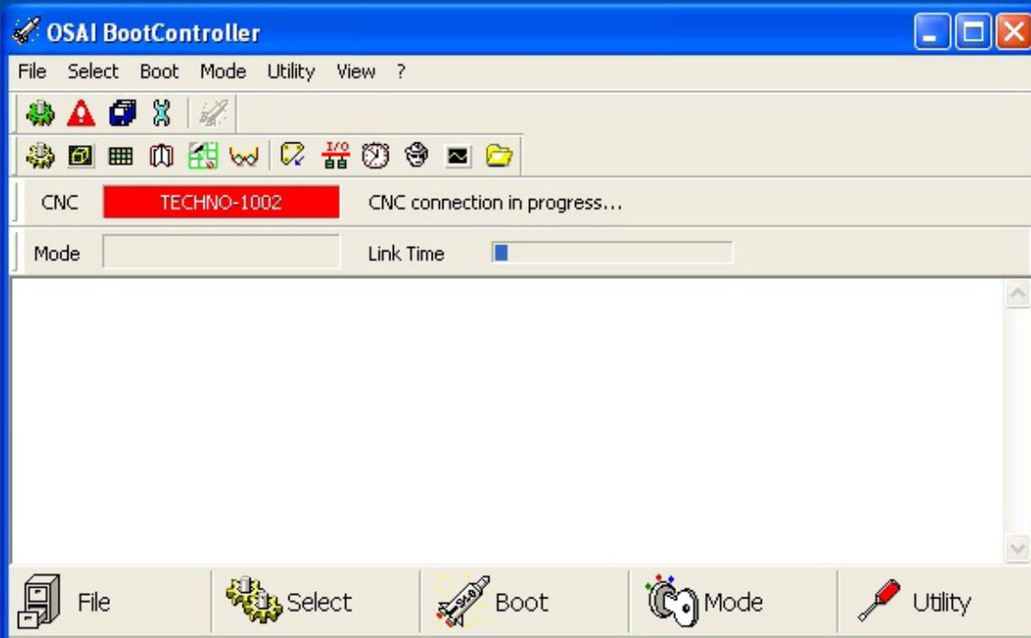
The Boot Controller software will start automatically. If it does not double click on the Boot Controller Icon on the desktop. If no text appears in the box, after 30 seconds, check that the light for the controller is on and that the network cable from PC to Osai controller is connected.
