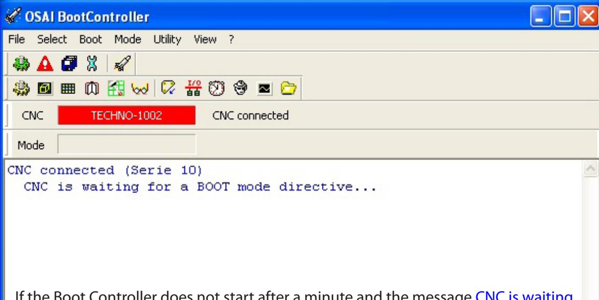
If the Boot Controller does not start after a minute and the message **CNC is waiting for a BOOT mode directive...** appears on the screen then normal mode needs to be selected. Click on the Mode Icon and select **Normal**.
