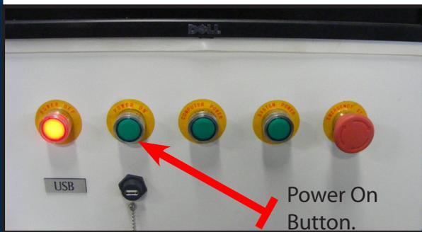
The red light on the front of the machine will light up, this indicates that 220 volts is coming into the machine.
