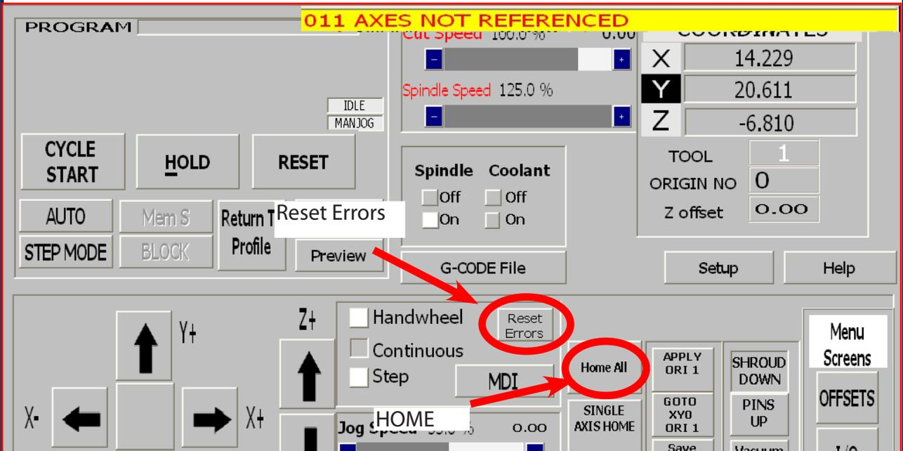
The **Axis not referenced** error will appear. Click on Home and all the axes will move to their home position. If any errors remain on the screen (i.e. **Low Air Pressure**), rectify the problem and click on Reset Errors to remove the message. The machine is now ready to be jogged.
