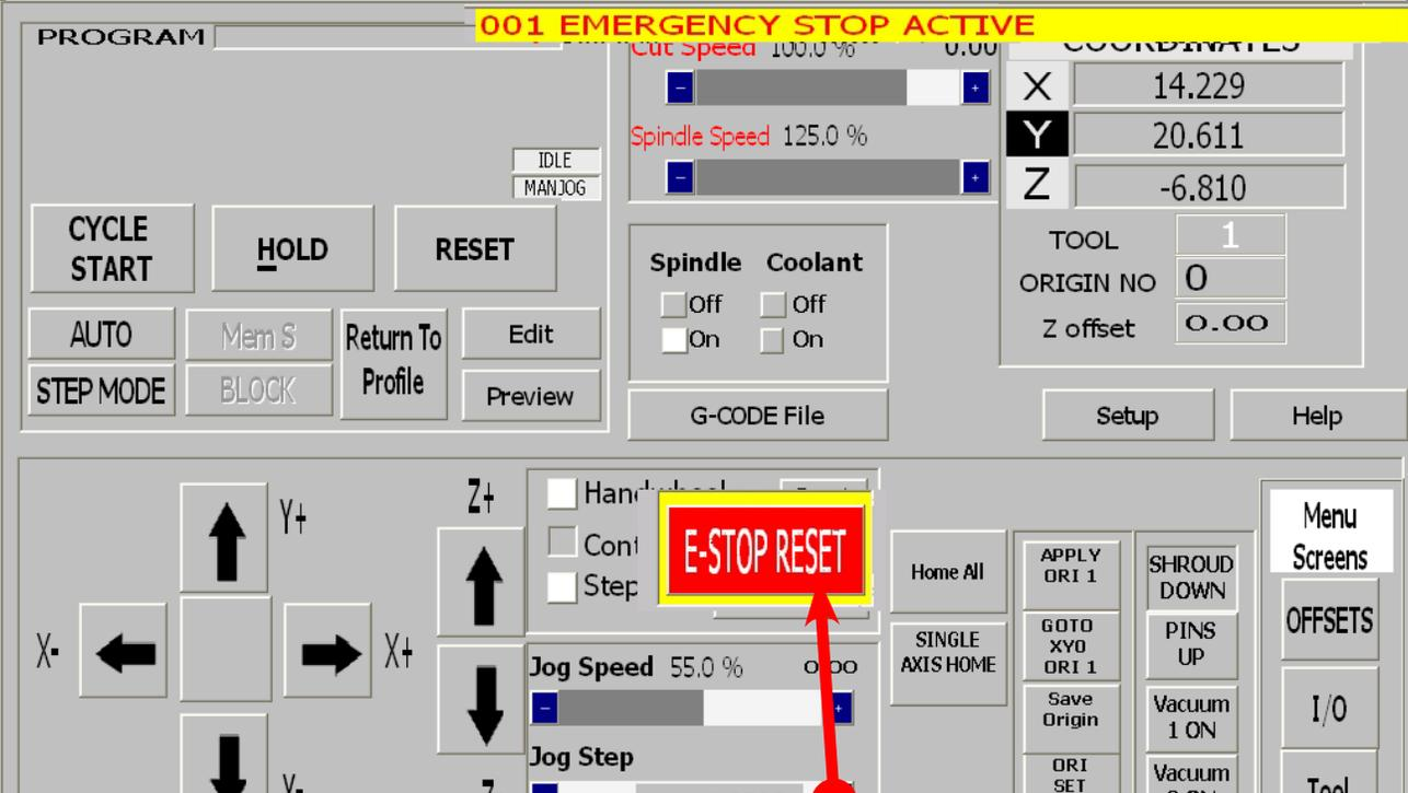
The Techno interface screen will now open. There will be a warning message saying **Emergency Stop Active**. Click on the E-stop Reset Button to remove this warning.
