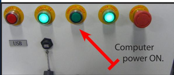
The Power on and System power light will light up indicating that power has been applied to the controller system and the motors. Press the Computer Power button to start the PC. This will only light temporarily.
