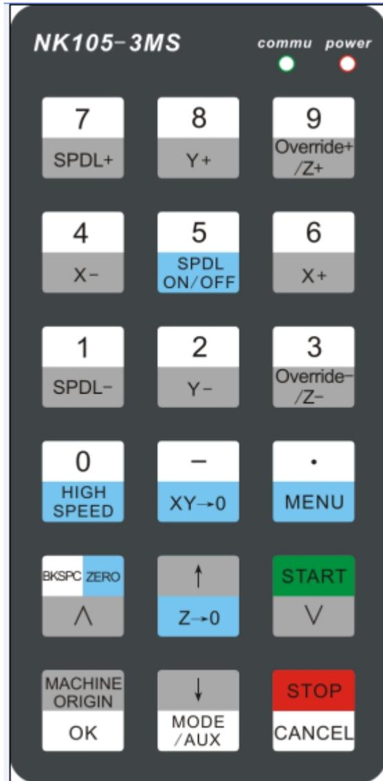
Fig. 4-2 Panel keys arrangement picture
