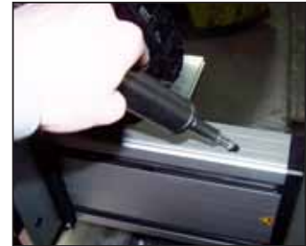
PICTURE 3A: Z-Axis Grease Fittings
