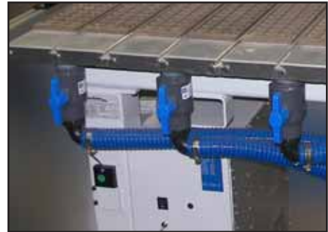
PICTURE 20: Vacuum Table Fixturing
