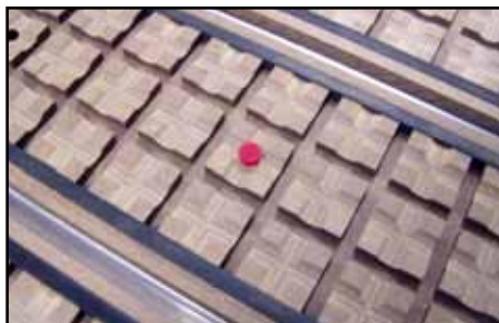
PICTURE 18: Foam Gasketing in Vac Table
