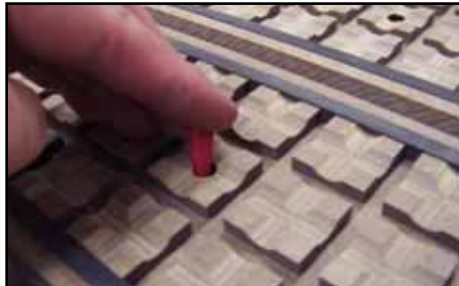
PICTURE 17: Rubber Plug in Vac Table
