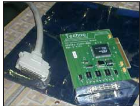
PICTURE 3: PCI Interface Card & SCSII Cable
