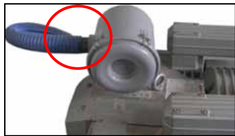
PICTURE 16: Filter-Vacuum Hose Conn.
