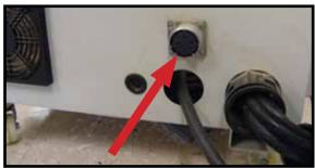
Attach the silver connector from the starter box here.
