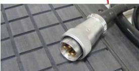
Take the Silver connector from the Starter Box and connect it to the female connector on the main electronic unit.
