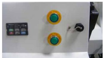
When the machine is powered on press the green button to turn the vacuum motor on and off.
