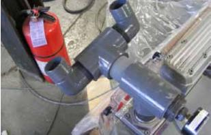
Attach the hoses from the machine to the T-connectors and attache them to the pump.
