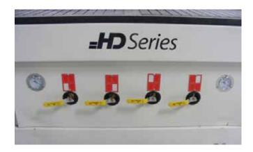
Turn on individual sections of the vacuum table by turning the manifold handles in the front of the machine.
