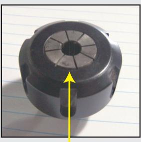
The picture above is how your collet nut assembly should look: the end of the collet is flush with the bottom surface of the collet nut. You will hear and feel a "SNAP" as the collet properly goes into the collet nut. Once it is assembled, then "SCREW" the nut onto the threaded spindle end.
